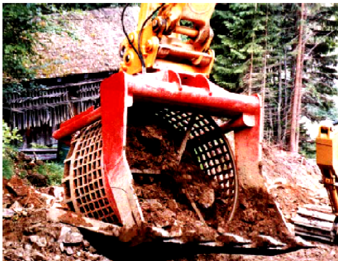
Screening adapter (for recycled material)
