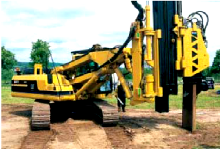
Sheet-wall piling equipment
