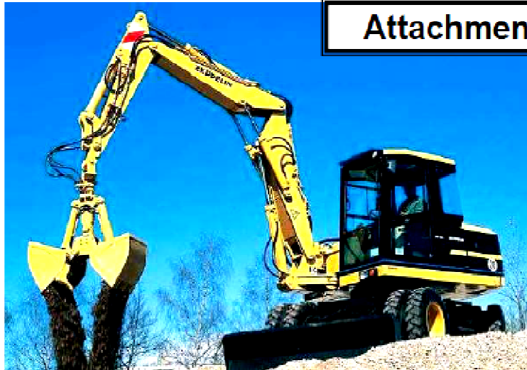
Clamshell bucket (for granular material)
