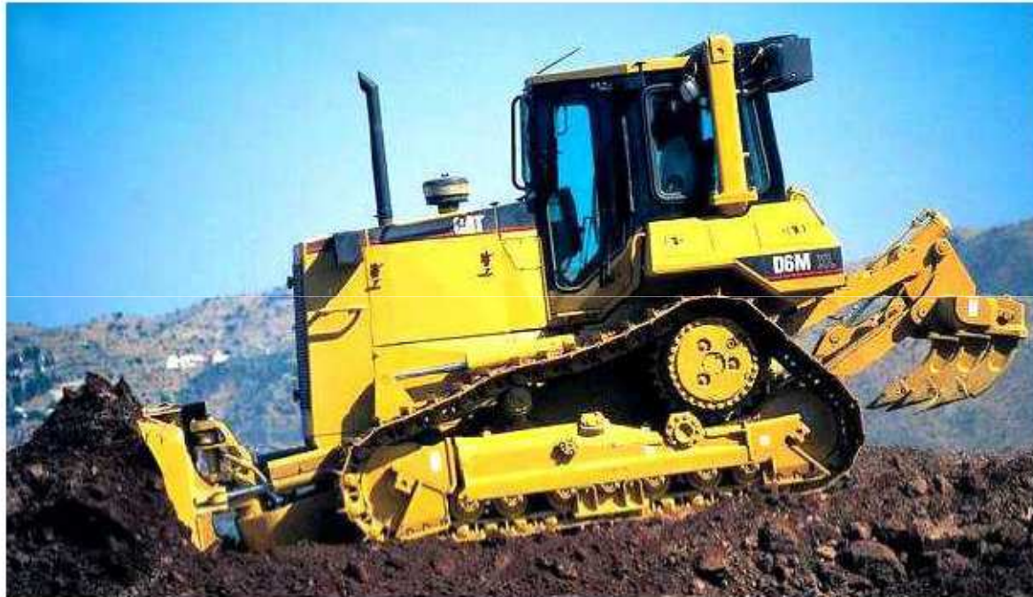
Bulldozer equipped with ripper attachment
