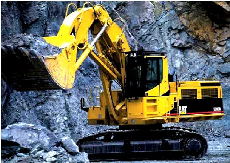
Front shovel, track-mounted
