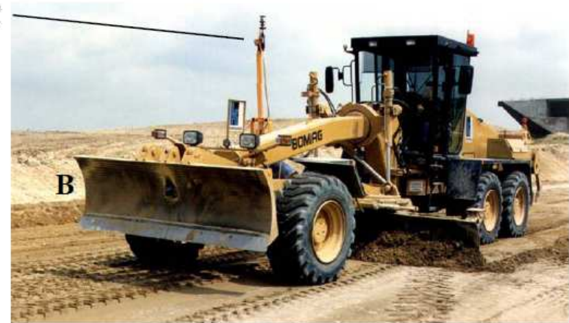
Laser controlled (C) grader equipped with ripper (A) and front blade (B) attachment
