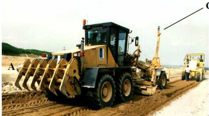
Laser controlled (C) grader equipped with ripper (A) and front blade (B) attachment
