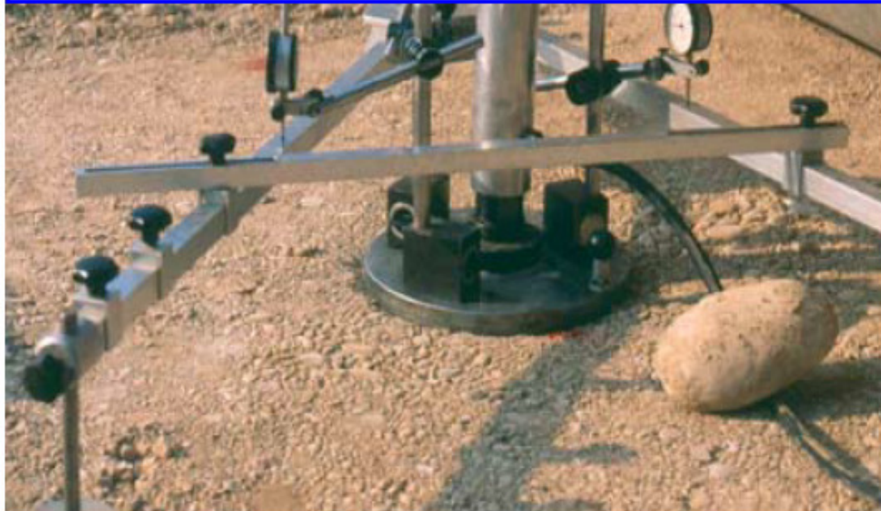
Static load plate test
