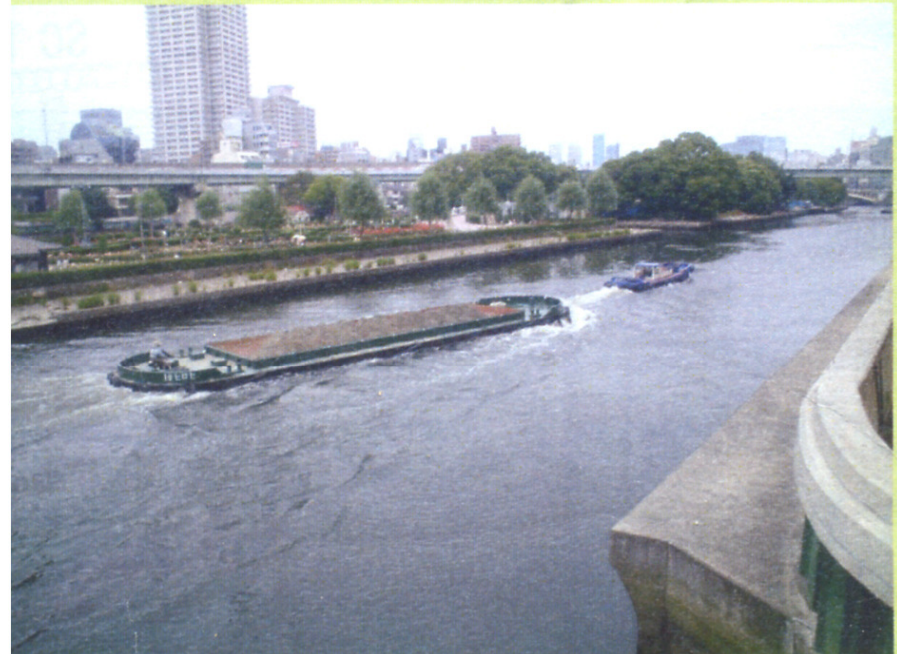
Spoil Transportation By the Hopper Barge
