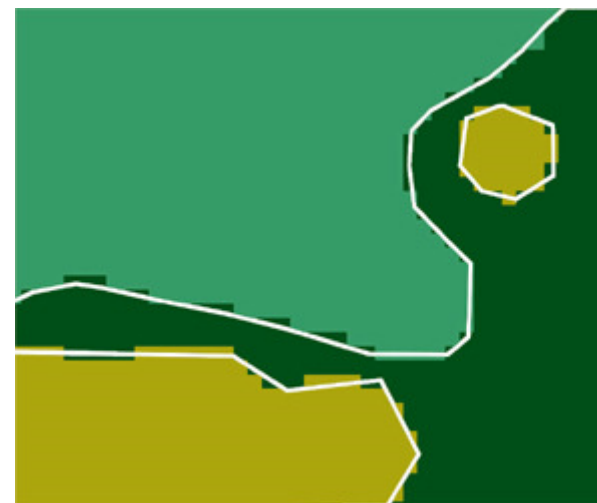
Figure 13b. Magnified views of the same GIS data file. converted into vector format.
