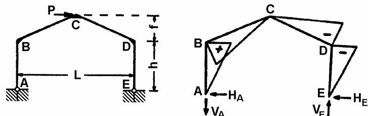
$$M_B = -M_D = +\frac{Ph}{2} \quad M_C = 0 \quad H_A = -H_E = -\frac{P}{2} \quad V_A = -V_E = -\frac{Phm}{L}$$
