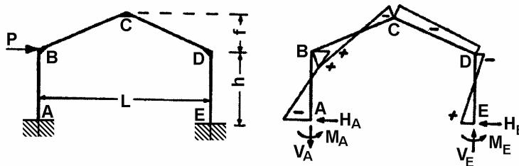
$$X_1 = \frac{3Pf(k + 2\phi k + \phi)}{2N_1} \quad X_2 = \frac{3Pfmk}{N_1} \quad X_3 = \frac{PhB}{2N_2}$$
