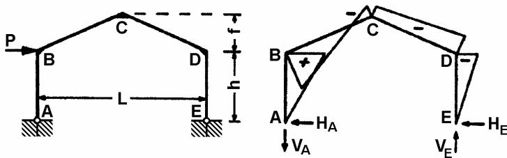
$$M_D = -\frac{Ph(B+C)}{2N} \quad M_B = Ph + M_D \quad M_C = \frac{Ph}{2} + m M_D$$
