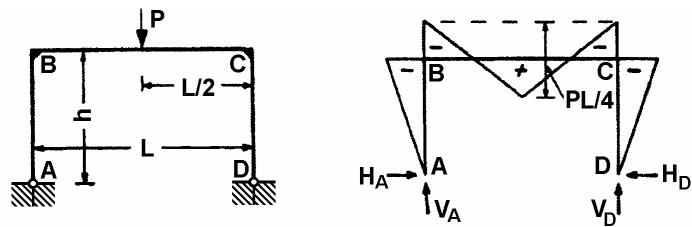
$$M_B = M_C = -\frac{3PL}{8N} \quad H_A = H_D = \frac{-M_B}{h} \quad V_A = V_D = \frac{P}{2}$$
