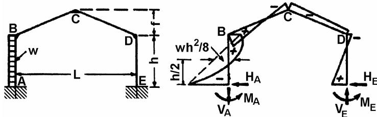
$$X_1 = \frac{wh^2}{8} \cdot \frac{k(k + 6) + k\phi(15 + 16\phi) + 6\phi^2}{N_1} \quad X_2 = \frac{wh^2k(9\phi + 8\phi^2 - k)}{8N_1} \quad X_3 = \frac{wh^2(2k + 1)}{2N_2}$$
