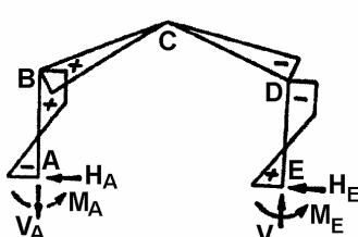
$$X_1 = \frac{Pa(B + 3b_1 k)}{N_2} \quad M_A = -M_E = -X_1 \quad M_B = -M_D = Pa - X_1 \quad M_C = 0$$
