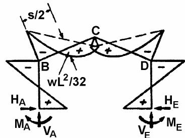
$$M_A = M_E = \frac{wL^2}{16} \cdot \frac{k(8+15\phi)+\phi(6-\phi)}{N_1} \quad M_B = M_D = -\frac{wL^2}{16} \cdot \frac{k(16+15\phi)+\phi^2}{N_1}$$
