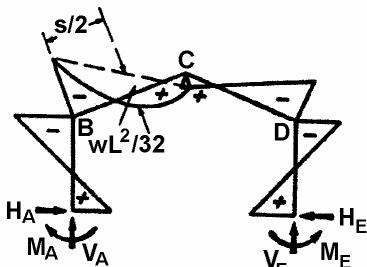
$$X_1 = \frac{wL^2}{32} \cdot \frac{k(8+15\phi)+\phi(6-\phi)}{N_1} \quad X_2 = \frac{wL^2}{32} \cdot \frac{k(16+15\phi)+\phi^2}{N_1} \quad X_3 = \frac{wL^2}{32N_2}$$
