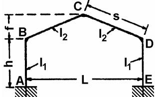
$$k = \frac{I_2}{I_1} \cdot \frac{h}{s} \quad \phi = \frac{f}{h} \quad m = 1 + \phi$$
