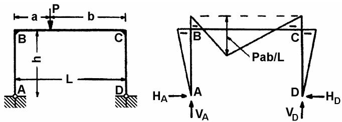
$$M_B = M_C = -\frac{Pab}{L} \cdot \frac{3}{2N} \quad H_A = H_D = \frac{-M_B}{h} \quad V_A = \frac{Pb}{L} \quad V_D = \frac{Pa}{L}$$
