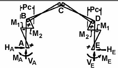
$$a_1 = \frac{a}{h} \quad b_1 = \frac{b}{h} \quad Y_1 = P c [2\phi^2 - (1 - 3b_1^2)k] \quad Y_2 = P c [\phi C + (3a_1^2 - 1)k]$$
