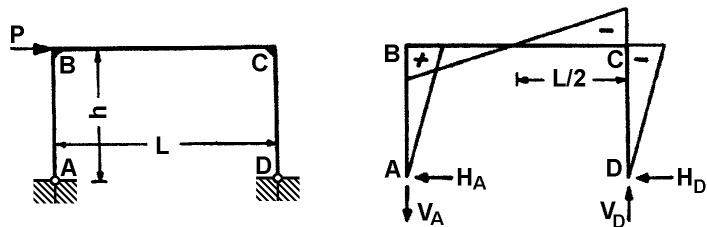
$$M_B = -M_C = +\frac{Ph}{2} \quad H_A = H_D = -\frac{P}{2} \quad V_A = -V_D = -\frac{Ph}{L}$$
