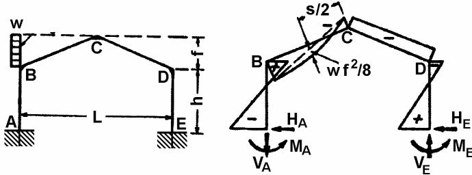
$$X_1 = \frac{wf^2}{8} \cdot \frac{k(9\phi + 4) + \phi(6 + \phi)}{N_1} \quad X_2 = \frac{wf^2}{8} \cdot \frac{k(8 + 9\phi) - \phi^2}{N_1} \quad X_3 = \frac{wfh}{8} \cdot \frac{4B + \phi}{N_2}$$
