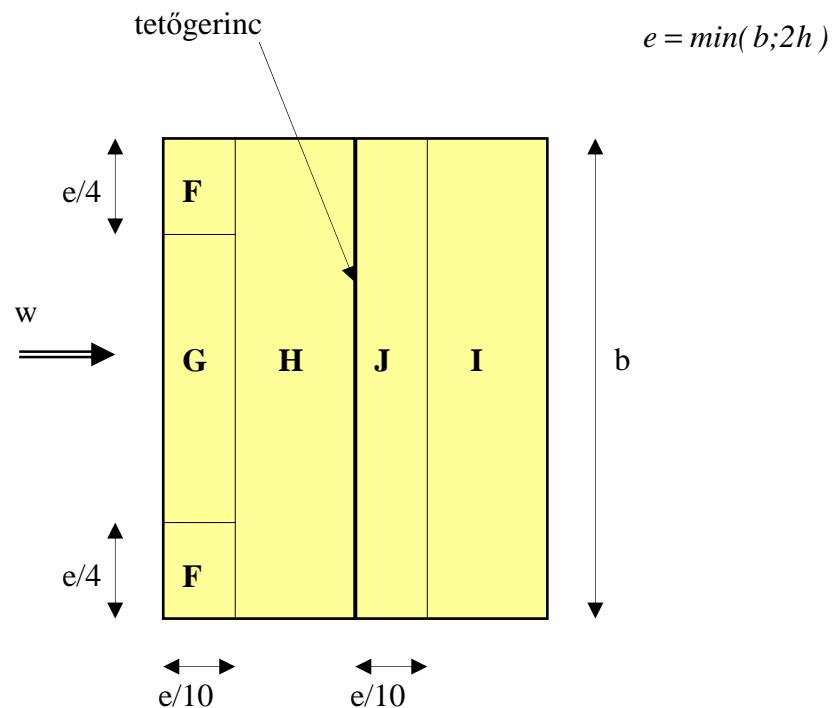
Annex 3: wind pressure on roof by longitudinal wind ( $\theta=90^\circ$ )
