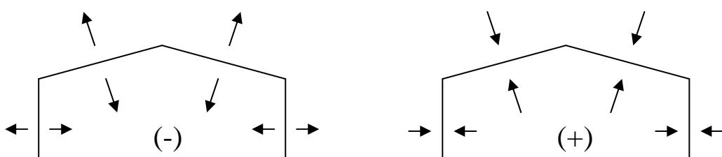
Both the external and internal reference heights for symmetric pitch roof which is not higher than the span of the building is equal to the height of the top point of the roof.
