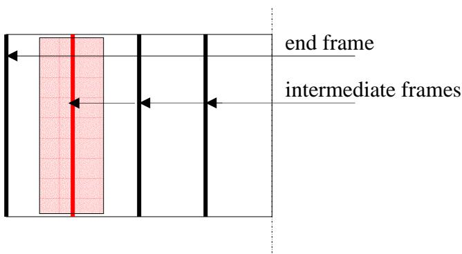
The main wind load cases for the intermediate frame (example for  $h/d < 0,25$ ,  $\alpha = 5^\circ$  and  $A > 10m^2$ ):
