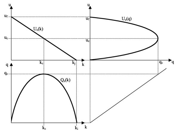
u - speed, u<sub>f</sub> - free speed, u<sub>c</sub> - critical speed, k - traffic density, k<sub>c</sub> - critical density, k<sub>j</sub> - maximum density, q - traffic volume, q<sub>c</sub> - maximum volume
