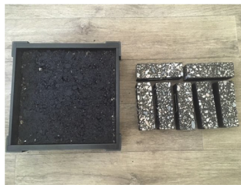
Fig. 2. Asphalt concrete samples: in the shape of a square slab with dimensions 305 \times 305 \times 50 mm (left); in the shape of a rectangular prism with dimensions 5 \times 5 \times 50 mm (right).
