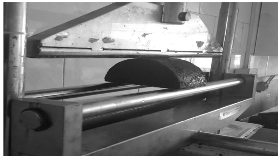
Fig. 6. Three-point bending test on a semi-cylindrical sample.
