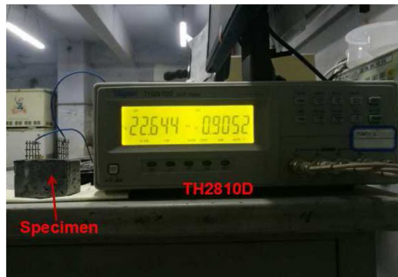
Fig. 1. Electrical resistance measurement.
