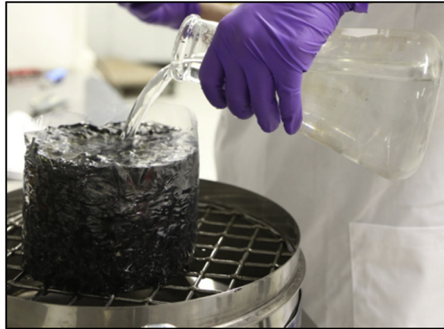
Fig. 4. Infiltration Rate Testing in Laboratory.
