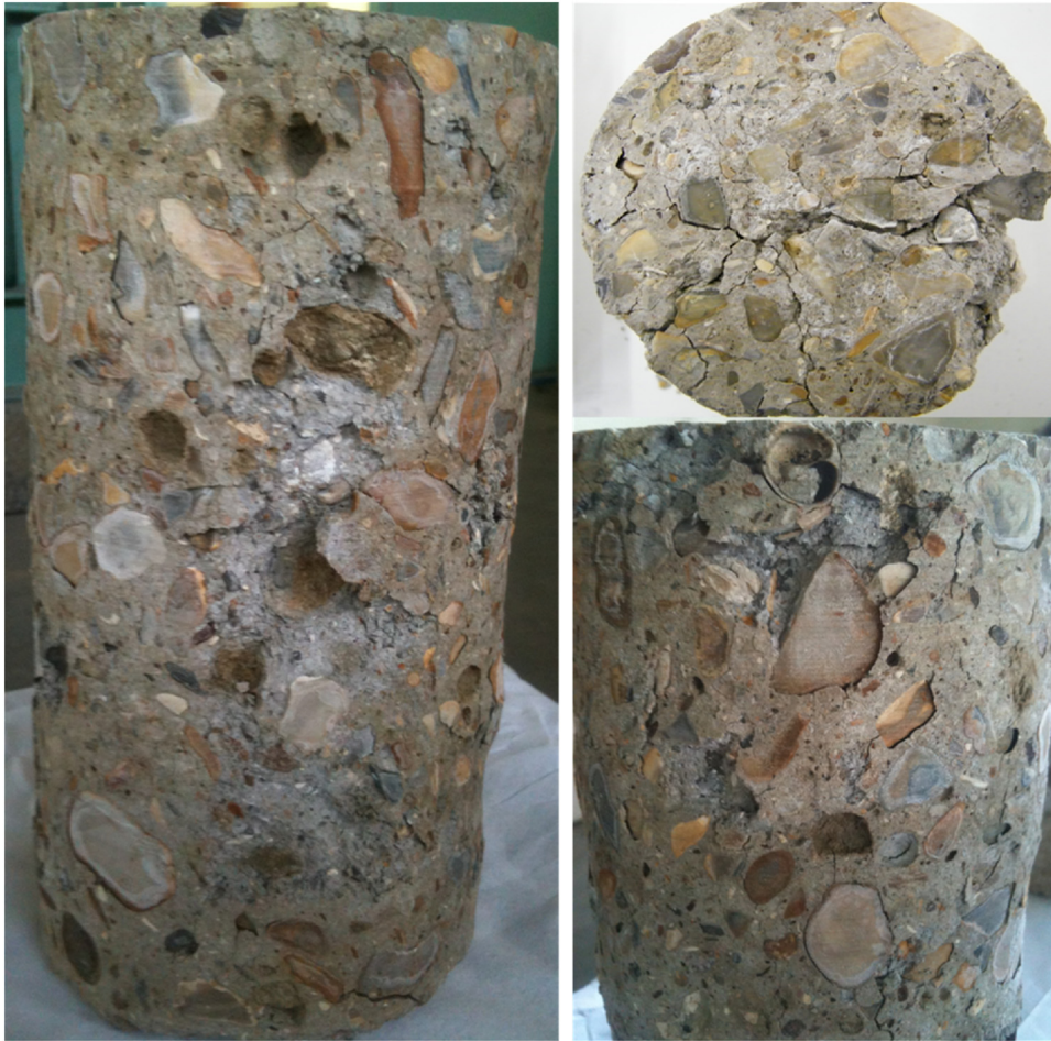
Fig. 15. Total degradation of C2 after three months of immersion/drying cycles at 105 °C.
