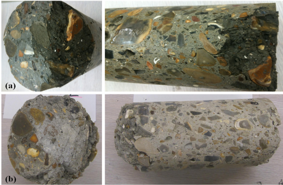
Fig. 9. Sample of C2 type concrete after (a) 58 cycles and (b) 85 cycles of freeze/thaw.
