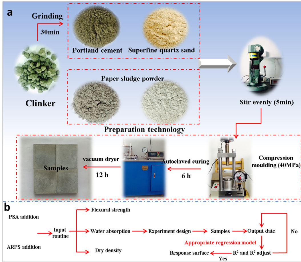
Fig. 3. (a) Flow chart of the fabrication and characterization of the CSBM and (b) the schematic diagram of RSM.
