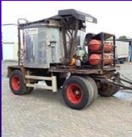
Mastic Asphalt cooker and using its product for bridge repair
