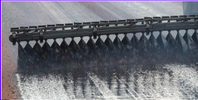
R-1 Aggregate Chip Spreader on road.mp4
