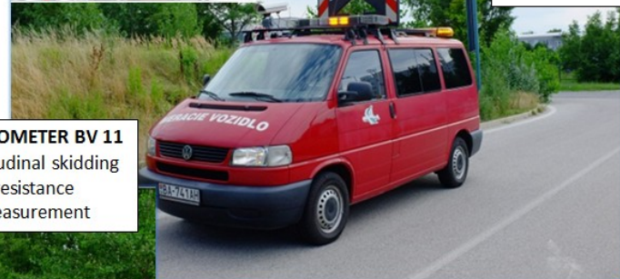
VIDEOCAR Quick visual inspections of pavement surface
