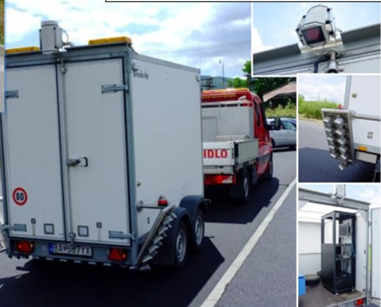
LINESCAN recording of pavement surface defects
