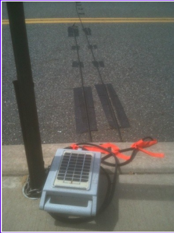
Pneumatic (rubber) traffic counting Tubes laid across the road surface
