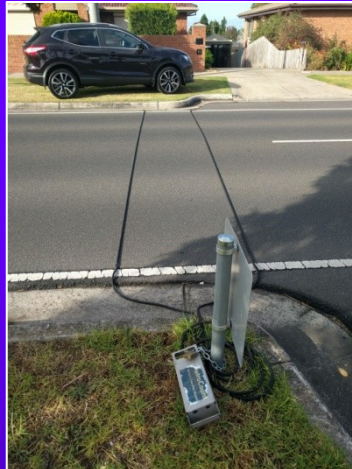
Pneumatic (rubber) traffic counting Tubes laid across the road surface
