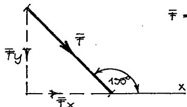
$$F = 5 \text{ kN} \quad \alpha = 225^\circ \quad 270^\circ - 225^\circ = 45^\circ$$
