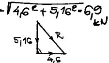
$$\begin{aligned} y_R &= 3 \cdot \frac{5.16}{4.6} = 3.37 \\ \tan \alpha &= \frac{3.37}{3} \\ \alpha &= 48.3^\circ \end{aligned}$$
