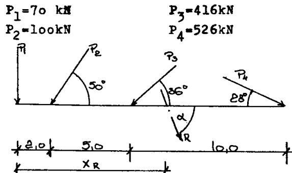
$$\begin{aligned} P_{1x} &= 70 \cdot 0 &= 0 \\ P_{2x} &= -100 \cos 50^\circ = -64,4 \\ P_{3x} &= -416 \cos 36^\circ = -338,0 \\ P_{4x} &= 526 \cos 28^\circ = 465,0 \end{aligned}$$
