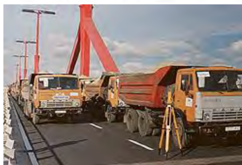
Figure 4.52 Load tests for the bridge.
