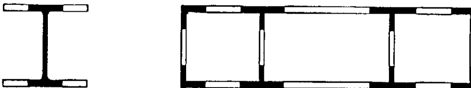
Figure 1.29 (a) Effective section (shaded) for typical members in axial compression.
