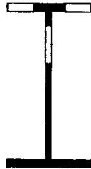
Figure 1.29 The application of effective widths of plate panels to determine effective cross-sections.
